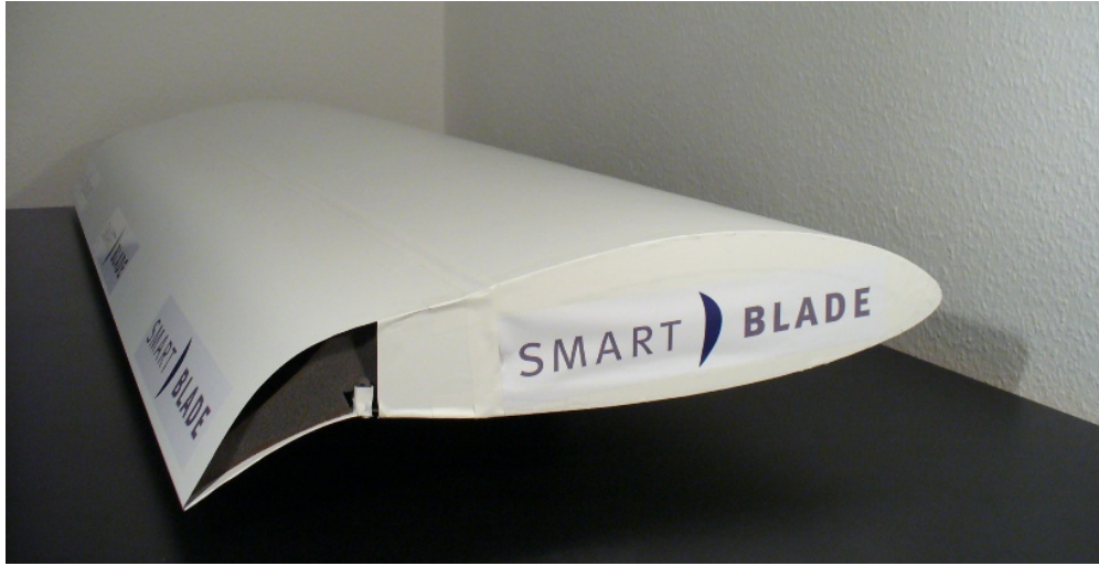
Figure 1: The test wing with the flexible flap mechanism extended at the fully extended positive position
